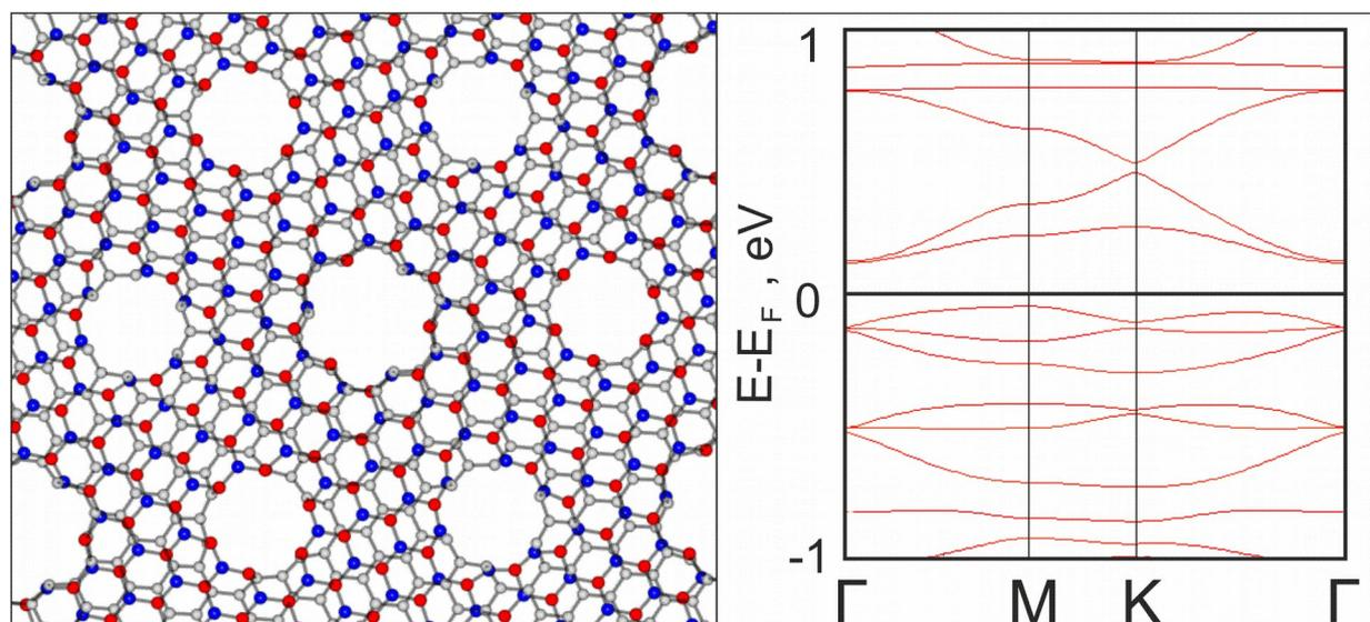
Fig. Semiconductor h-BN-graphene nanomesh and its band structure.  $E_g=0.18$  eV
